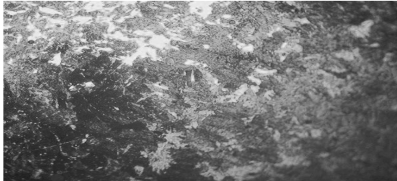
Plate 5: Weld Zone Microstructures (Water Cooled)
