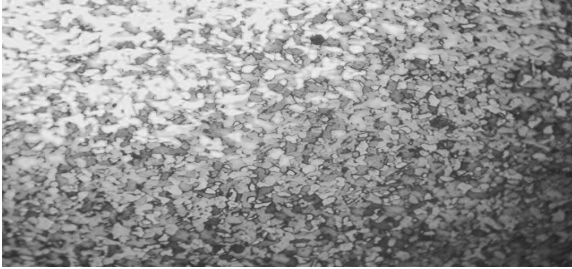
Plate 2: Weld zone and Heat Affected Zone (cooled under room temperature)
