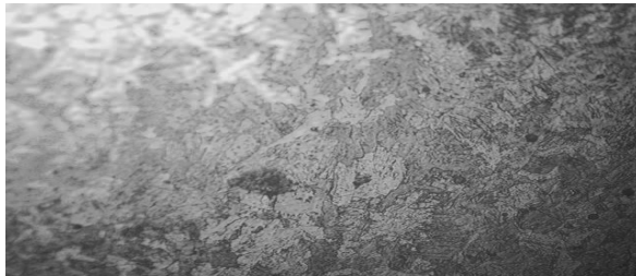
Plate 5: Weld Zone Microstructures (Water Cooled)
