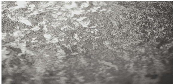
Plate 6: Weld Zone Microstructures (Salty Water Cooled)
