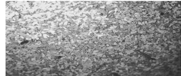
Plate 4: Heat Affected Zone (Salty Water Cooled)
