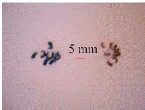
Fig. 9. Picture showing chips produced by a 2 mm depth of cut at 0.23 feed rate, and cutting speed of 190 m min -1 [7]
