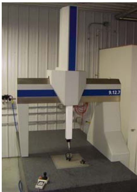
Fig. 6. Dimensional metrology using CMM
