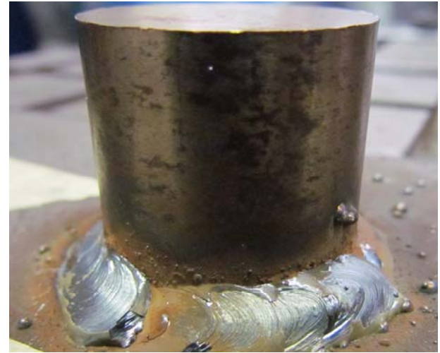
Fig. 3. Hand welded cap before robot milling
