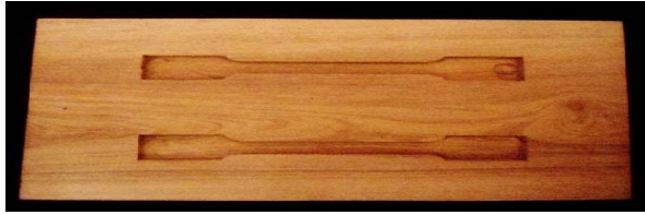
Fig. 6: Wooden Die block for tensile test
