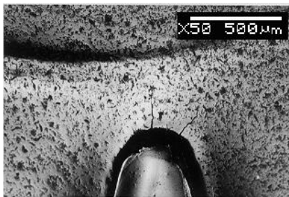
Fig. 5 Working surface of the testing die-casting die. Surface cracks and pits. OM.
