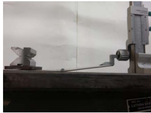
Fig. 3. Measurement of angular distortion
