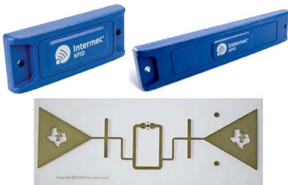
Fig. 3. IT65 small and large passive RFID tags and Texas Instruments Gen2 tag [15]
