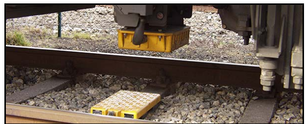
Fig. 2. A balise is placed on the line and a scanner is equipped under the locomotive [11]
