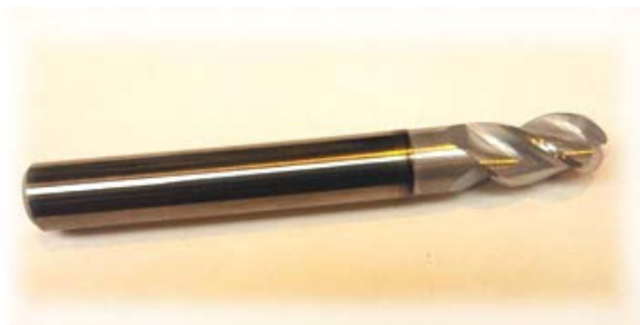
Fig. 2. Ball-nose end mill cutter used in machining
