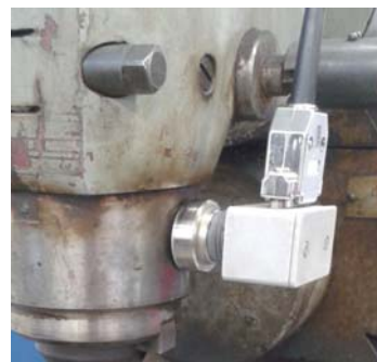
Fig. 3. Detail of the location and attachment of the sensor on the spindle head housing of the milling machine
