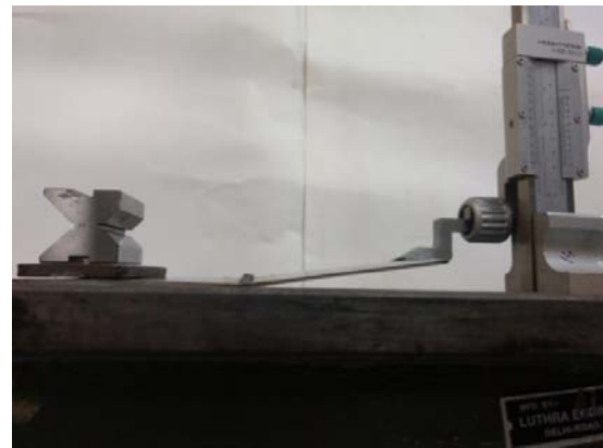
Fig. 3. Measuring the angular distortion
