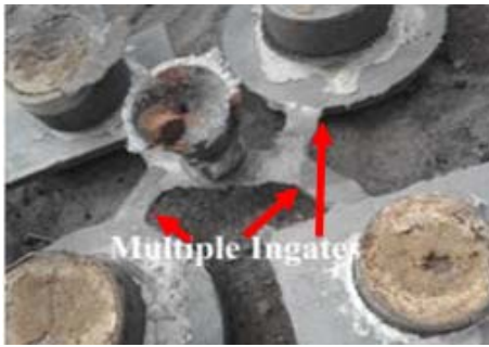
Fig. 12. Multi Gate System
