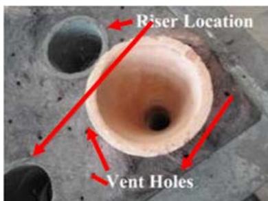
Fig. 2. Vent Holes and Riser Placing
